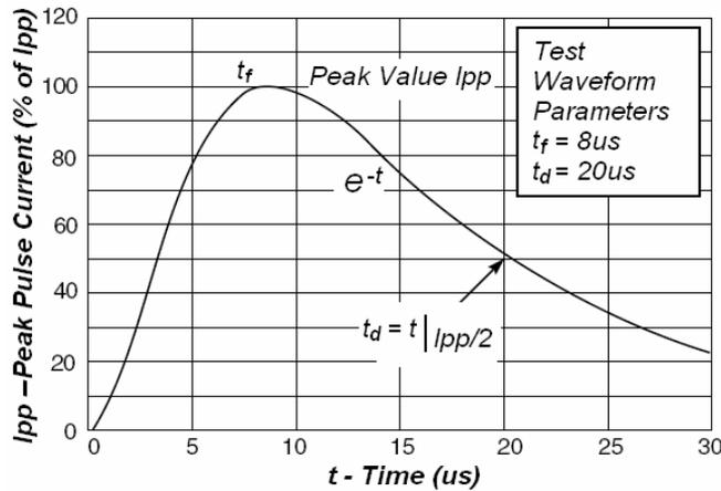
**Fig1. Pulse Waveform**
